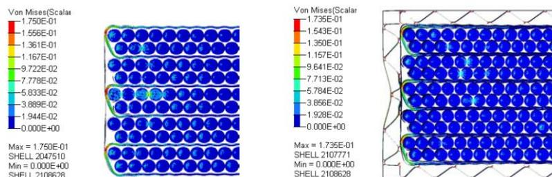
a) Von Mises stress results for the base model    b) Von Mises stress results for the shock absorber model
