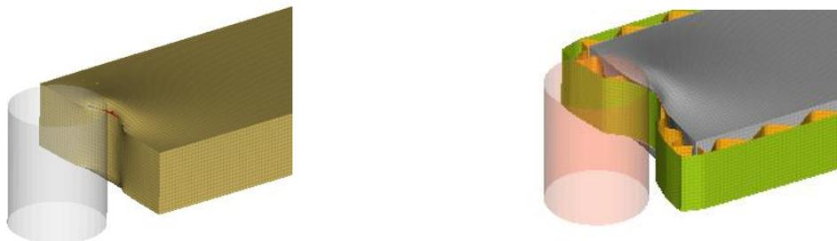
a) Deformation of the base battery pack at 21 m/s
