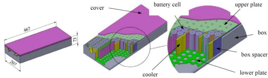
**Figure 1.** CAD model of battery pack
